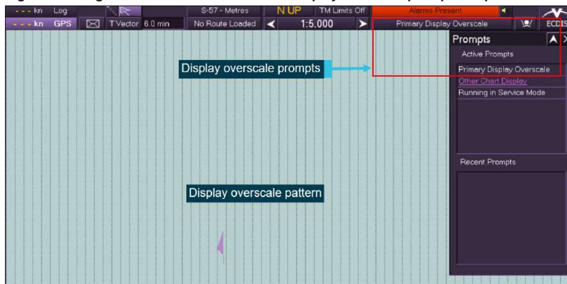
Figure 13: Image of a VisionMaster FT ECDIS display overscale prompt and pattern
