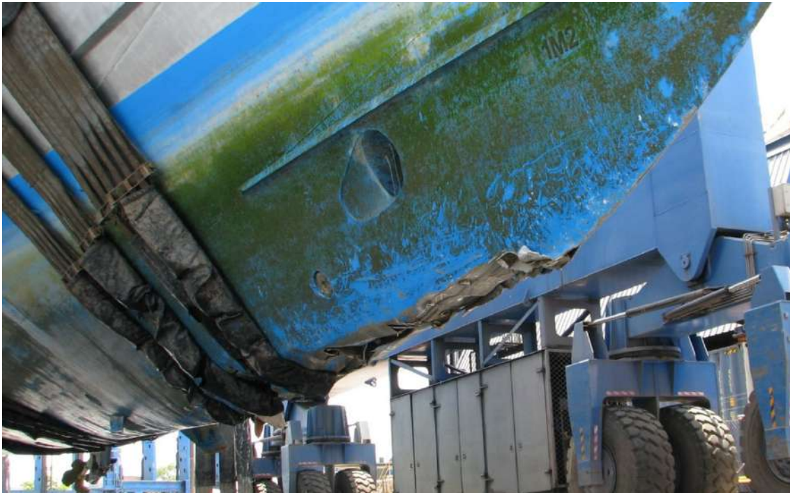
Figure 9: Damage to ABFC Roebuck Bay's keel
