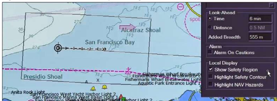
Figure 25: ECDIS look-ahead safety checking function
