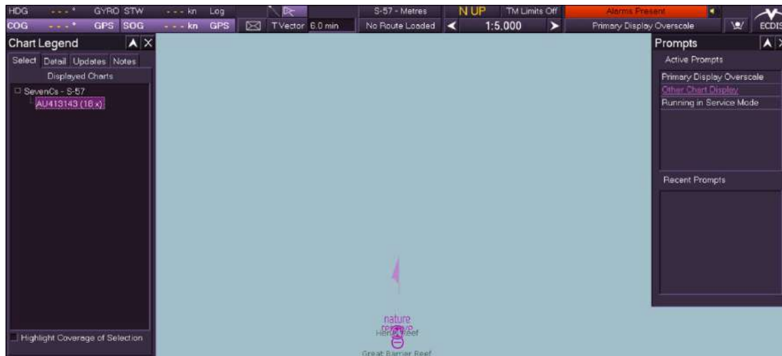
Figure 14: Image of ENC AU413143 showing no overscale pattern
