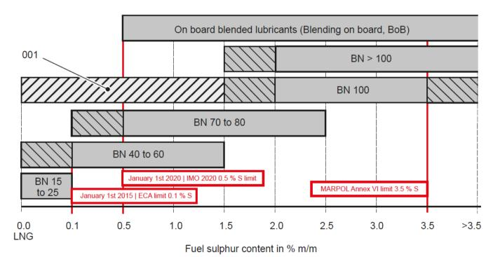
From the chart above, WIN G&D recommends the use of 40BN (Gulfsea Cylcare DCA 5040H) to 70BN (Gulfsea Cylcare DCA 5070H) cylinder oil for engines burning <0.5% Sulphur fuels. But if the condition of the engine is found unsatisfactory (for instance, cold corrosion or deposits build-up observed), a higher BN cylinder oil (Gulfsea Cylcare DCA 5070H) is recommneded.
