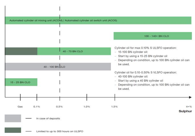
From the chart above, MAN recommends the use of 40BN cylinder oil (Gulfsea Cylcare DCA 5040H) for engines burning <0.5% Sulphur fuel. But if the condition of the engine is unsatisfactory (for instance, cold corrosion or deposits
